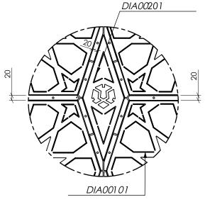
Use a rectangular grid measuring 631 by 600 to position panels in the correct alignment.
